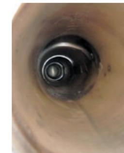
The lining has slightly discoloured, no blisters occur. The steel is not affected.
