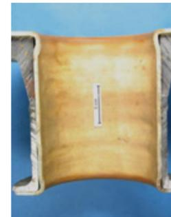
The lining has slightly discoloured, but no blisters occur. The steel material was not affected.
